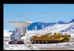
One of the Atacama Large Millimeter/submillimeter Array (ALMA) antennas stands next to Lore, the ALMA transporter. Lore moves antennas between Chajnantor and the lower altitude Operations Support Facility for maintenance
